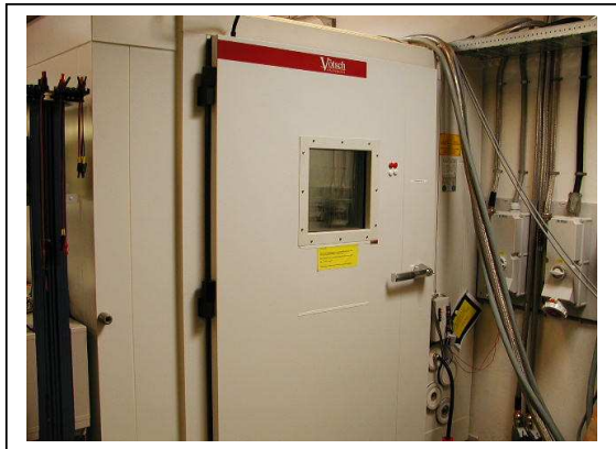
Picture from the damp head camber.
