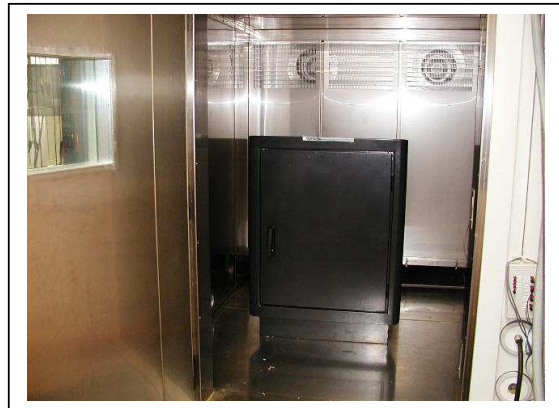
Picture from the damp head camber.
